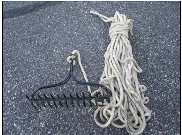
Figures 1 and 2. Double-headed, weighted garden rake, attached to a rope used to survey aquatic vegetation.
